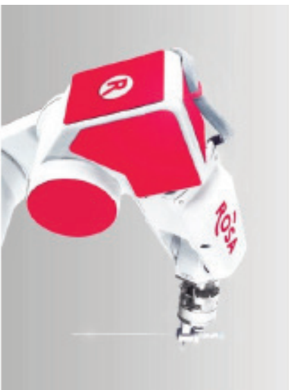
Robot guidance system allows neurosurgeons to precisely place electrodes deep in the brain for SEEG procedures to pinpoint where seizures arise.
